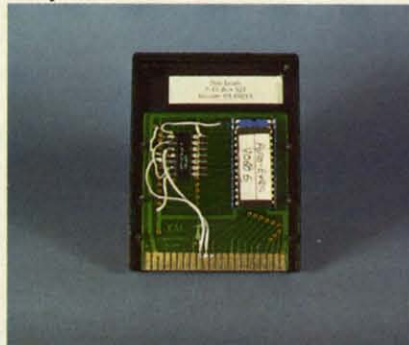
Turnkey 64 uses readily available ROM cartridge with control flip-flop added.
